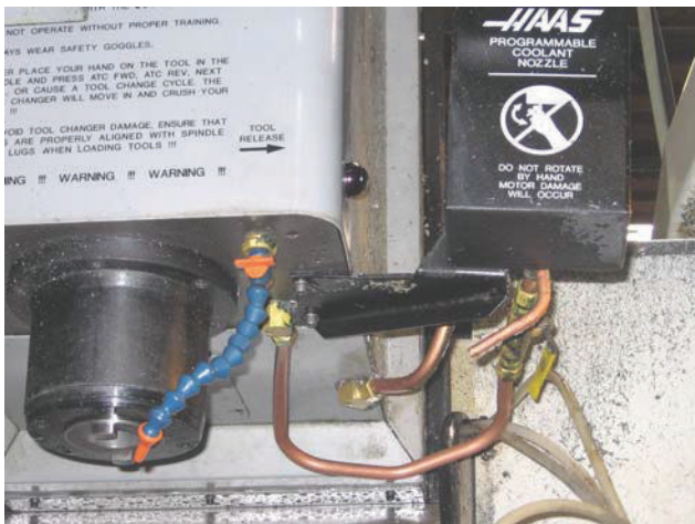
Figure 1. Typical old installation without coolant manifold
