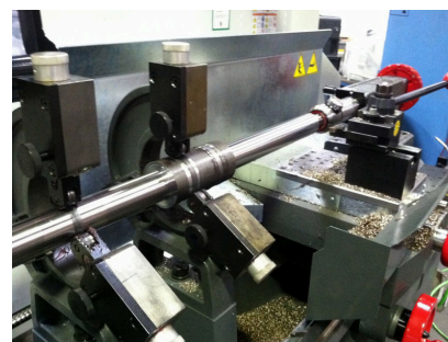
The above part was machined, using the M38 SSV feature
